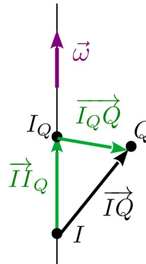
$$\begin{aligned} \overrightarrow{IQ} &= \overrightarrow{II}_Q + \overrightarrow{I}_Q\overrightarrow{Q} \\ \overrightarrow{II}_Q &\parallel \vec{\omega} \end{aligned}$$
