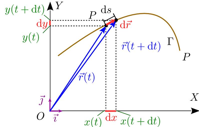
$$d\vec{r} = \vec{r}(t + dt) - \vec{r}(t) = dx \vec{i} + dy \vec{j}$$
