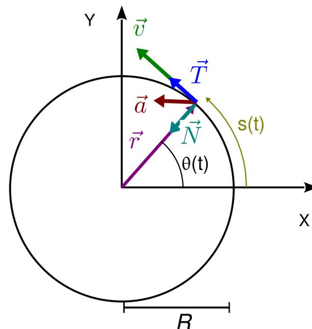
$$\begin{aligned} \vec{T} &= [-\sin \theta, \cos \theta, 0] \\ \vec{N} &= [-\cos \theta, -\sin \theta, 0] \\ \vec{B} &= [0, 0, 1] \end{aligned}$$
