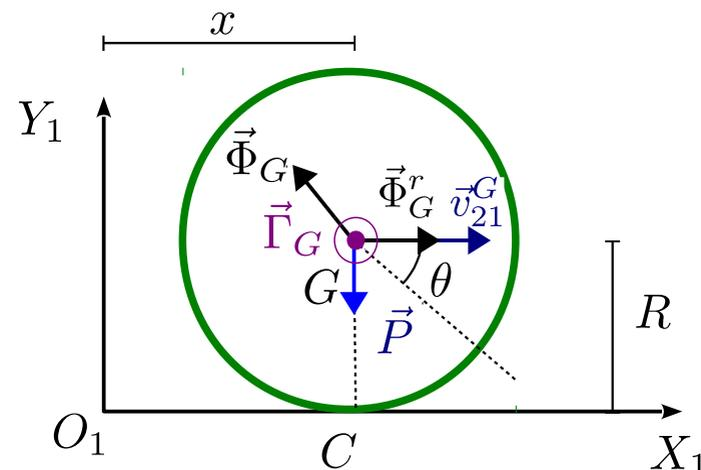
$$\Phi_x = -\frac{I}{R^2} \dot{v} \quad \Phi_y = P \quad \Gamma = -\frac{I}{R} \dot{v} \quad \Phi_r = \left( M + \frac{I}{R^2} \right) \dot{v}$$
