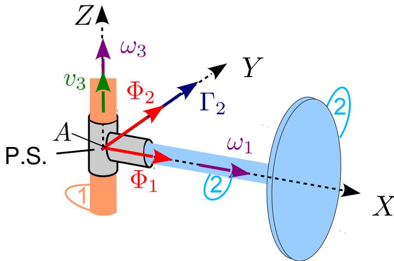
$$\vec{v}_{21}^A = [0, 0, v_3] \quad \vec{\omega}_{21} = [\omega_1, 0, \omega_3]$$
