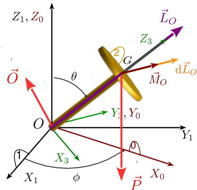
$$\begin{aligned} \vec{\omega}_{31} &= \vec{\omega}_{30} + \vec{\omega}_{01} \\ &= [-\dot{\phi} \operatorname{sen} \theta, \dot{\theta}, \dot{\phi} \operatorname{cos} \theta]_3 \end{aligned}$$
