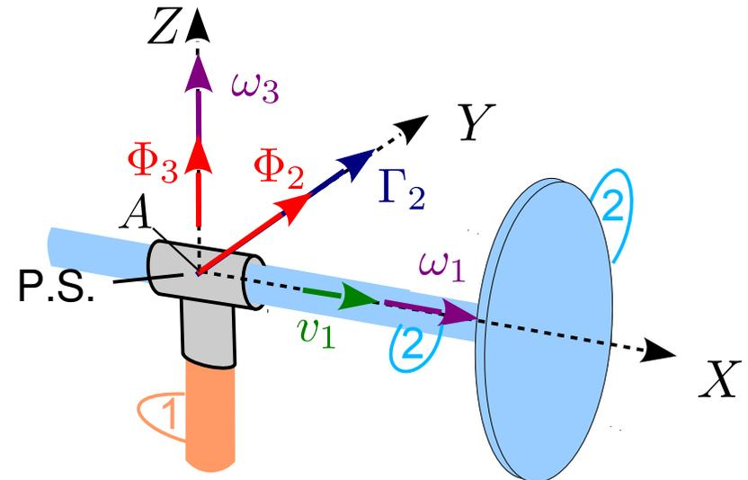
$$\vec{v}_{21}^A = [v_1, 0, 0] \quad \vec{\omega}_{21} = [\omega_1, 0, \omega_3]$$
