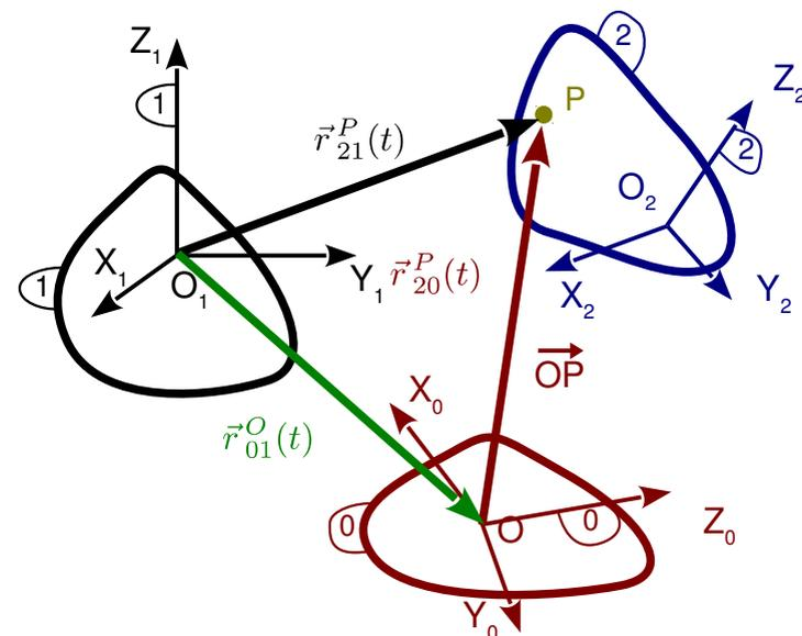
$$\vec{a}_{21}^P = \vec{a}_{20}^P + \vec{a}_{01}^P + 2\vec{\omega}_{01} \times \vec{v}_{20}^P$$
