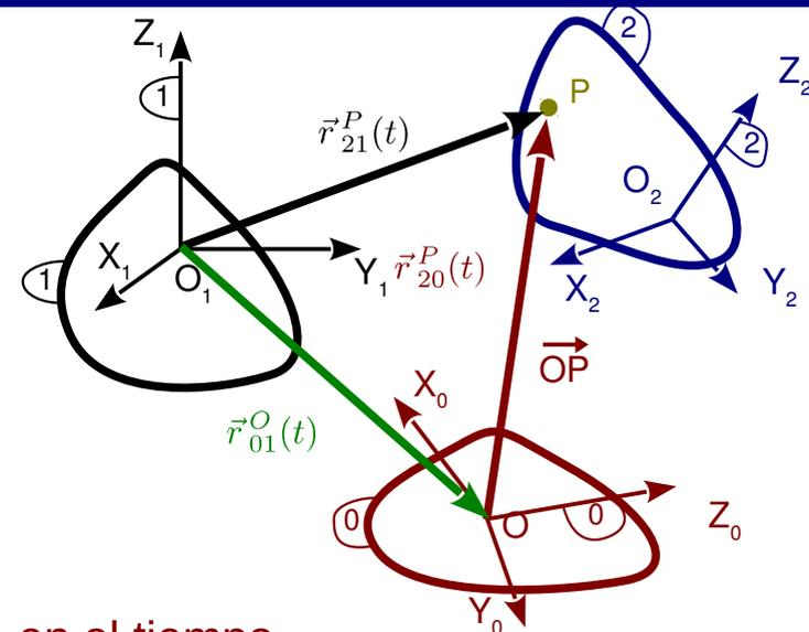
$$\left. \frac{d\vec{r}_{21}^P(t)}{dt} \right|_1 = \left. \frac{d\vec{r}_{01}^O(t)}{dt} \right|_1 + \left. \frac{d\vec{r}_{20}^P(t)}{dt} \right|_1$$
